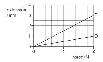
The wires have the same original length but different diameters.
